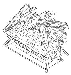
Figure 20 - Placement of Top Logs
